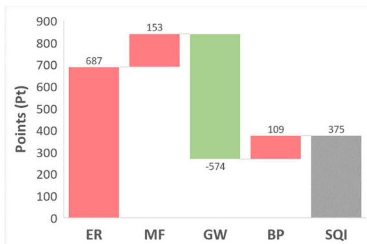
Figure 4 - Waterfall diagram of the four resized indicators, where ER represents erosion resistance, MF the mechanical groundwater filtering capacity, GW the groundwater recharge capacity, and BP the biotic (biological) production potential.
