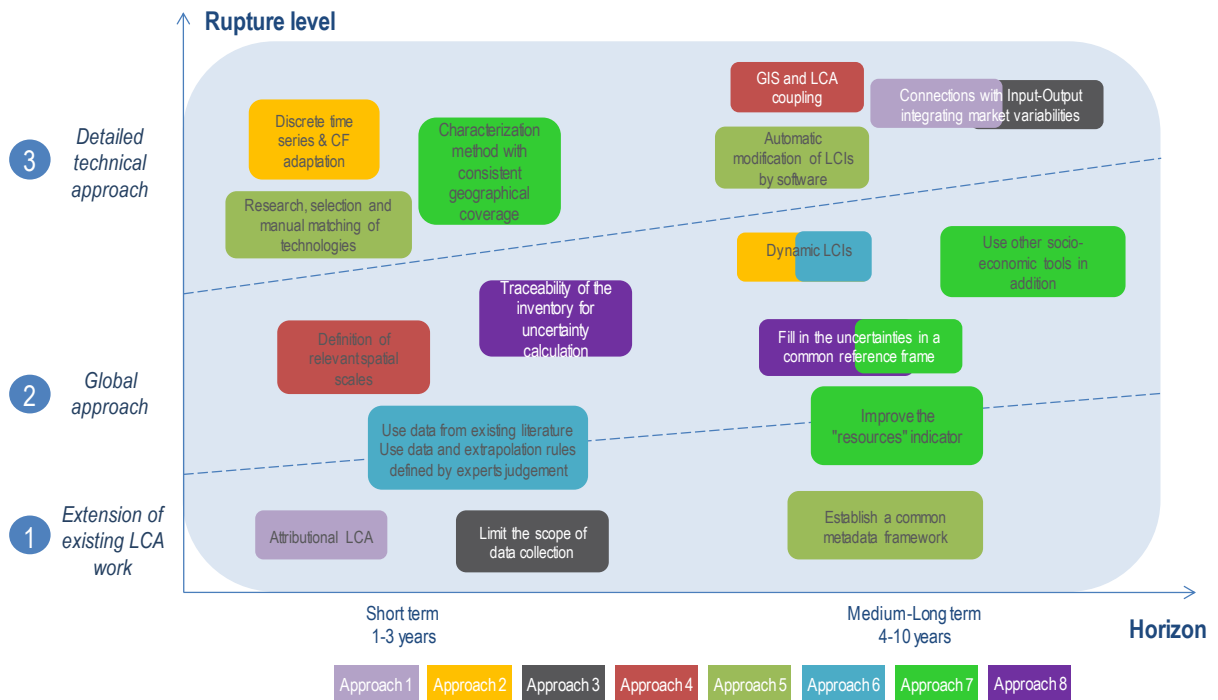
Figure 6 : Short- and medium-term research options for improving the LCA assessment of an energy transition scenario
